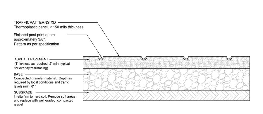
TYPICAL PAVEMENT WITH TRAFFICPATTERNS XD™ CROSS-SECTION DETAIL
